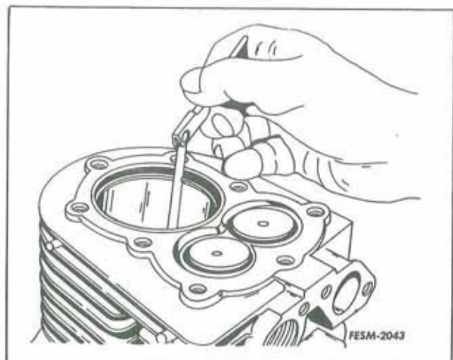
Illust. 1-9. Measuring ring gap.
