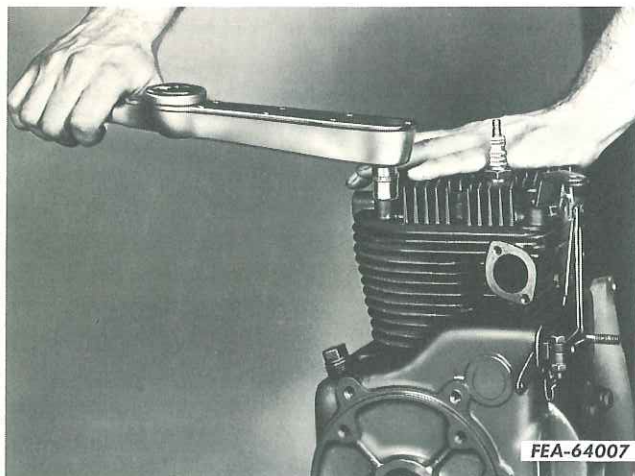
Illust. 18. Tightening cylinder head cap screws.
