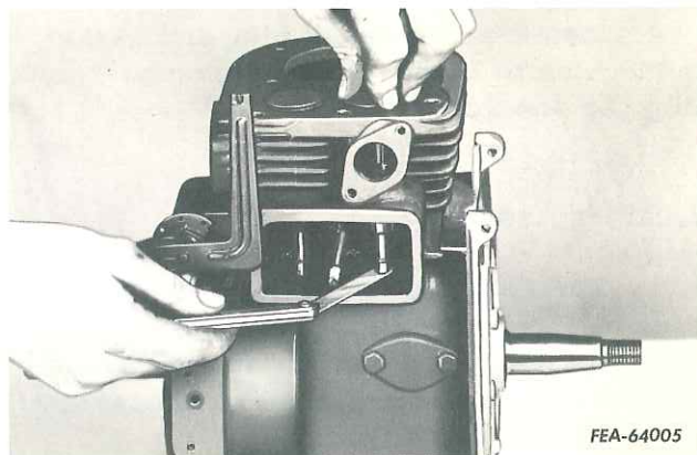
Illust. 16. Checking valve clearance.
