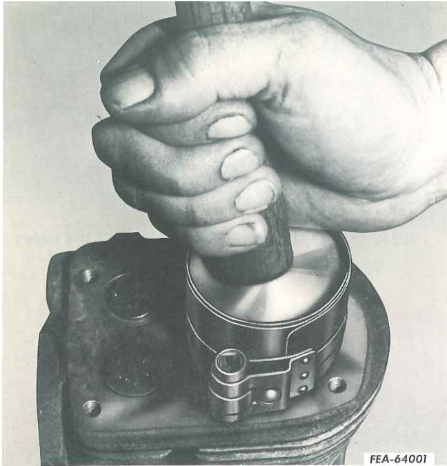
Illust. 12. Installing piston assembly.
