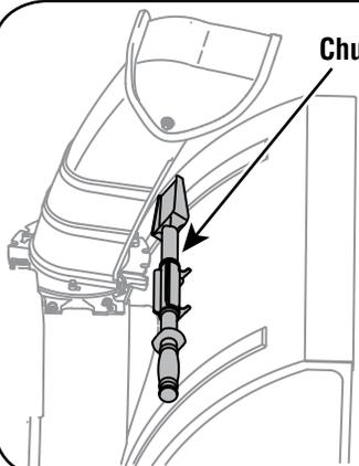
A chute clean-out tool is fastened to the top of the auger housing with a mounting clip. The tool is designed to clear a chute assembly of ice and snow.
