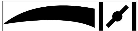
The choke control is found on the rear of the engine and is activated by rotating the knob clockwise. Activating the choke control closes the choke plate on the carburetor and aids in starting the engine.
