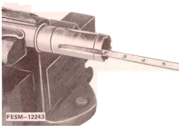
**NOTE:** Before removing the second bearing, measure the distance from the end of the shaft to the bearing. Record this measurement for reassembly purposes.
