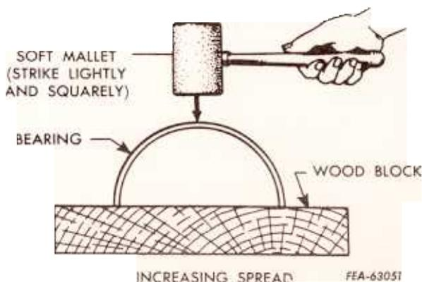
(b) **INSUFFICIENT SPREAD:** If measurement of bearing indicates insufficient spread, place bearing on a wood block and strike the back of the bearing lightly and squarely with a soft mallet. Recheck measurement and if necessary continue until correct width is obtained.
