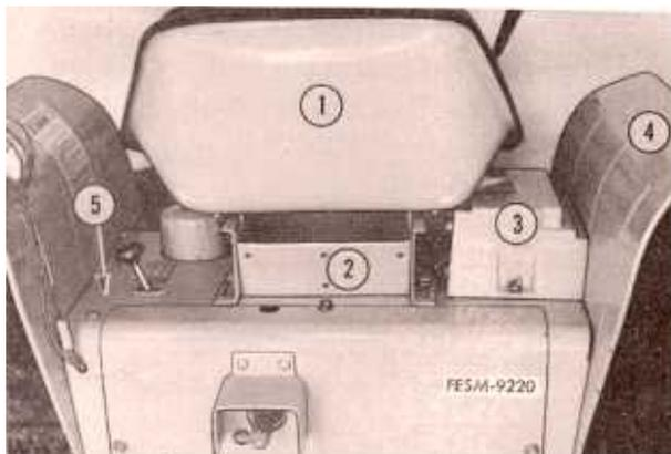
7. Remove the seat (1), and seat support assembly (2) as a unit.
