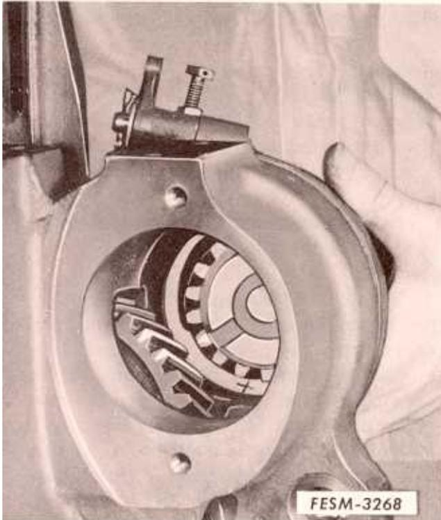
Install the governor assembly and ignition unit using new mounting gaskets, insure proper ignition timing as follows:
