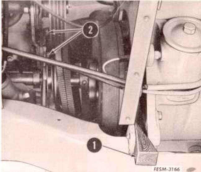
8. Remove six cap screws securing the engine to the frame (four in rear and two in front).
