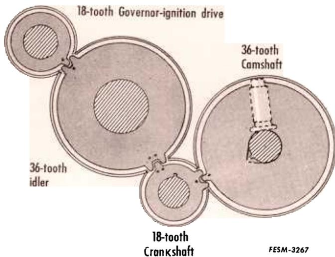
3. Install the key in the crankshaft if it was removed. Heat the crankshaft gear and install the gear, being sure the single timing mark of the camshaft gear and the single mark on the crankshaft gear are aligned.
