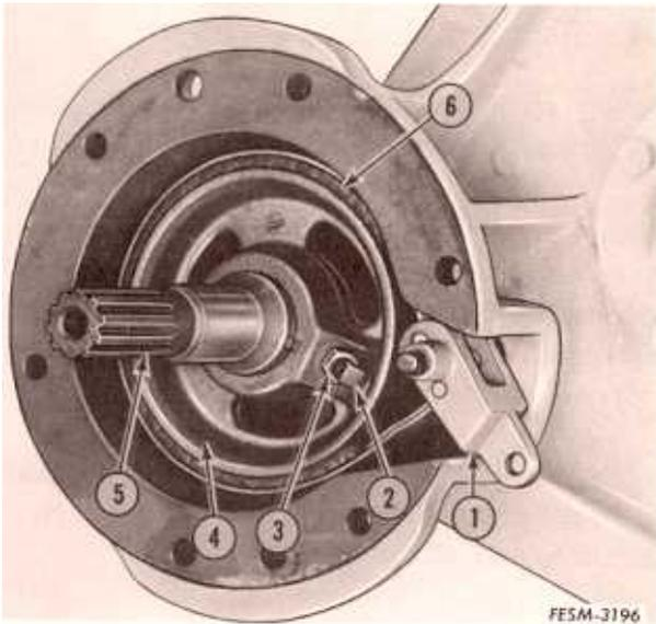
4. Align the brake drum keyway with the key on the differential shaft and install the brake drum (4) on the shaft (5). Tighten the set screw (2) and lock nut (3) securely.
