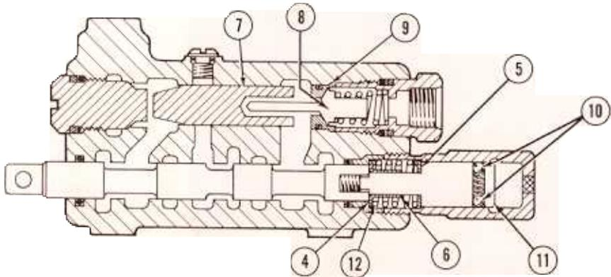
Hydraulic control valve cross section.
