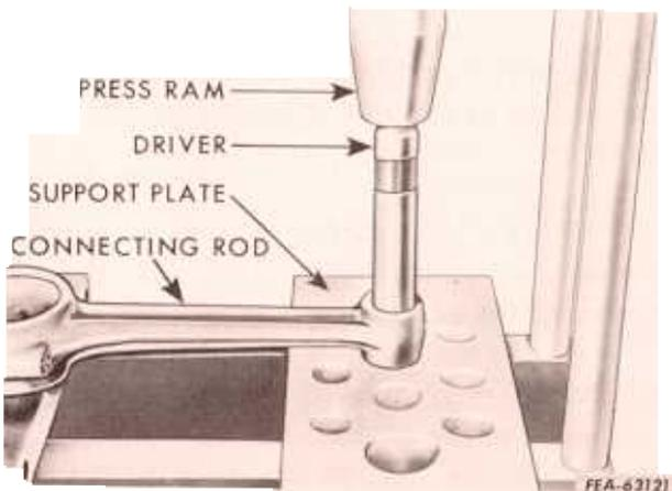
14. Align the new piston pin bushing on the connecting rod so that the oil hole in the bushing will match with the oil hole in the connecting rod. Press the bushing into the rod.
