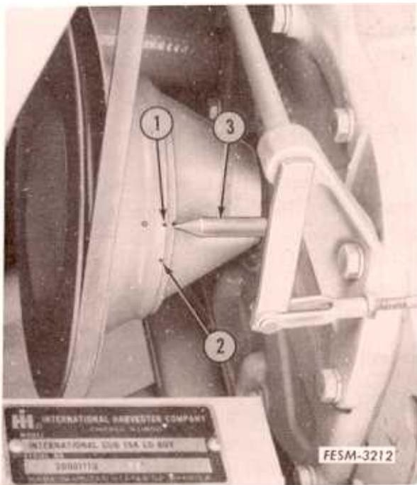
10. Place the number one spark plug cable in a position so that the spark to ground will be audible when hand cranking the engine. Then advance or retard the ignition distributor until spark occurs as the O mark (1) on the fan drive pulley aligns with pointer (3) while hand cranking engine.
