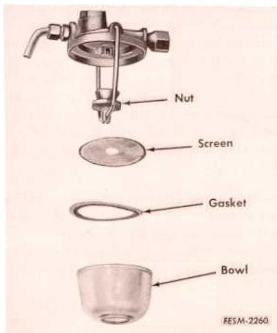
After the dismantled parts have remained in the solvent long enough to dissolve the coatings, remove and rinse in petroleum base cleaning solution. Dry all parts with compressed air, blowing through all jets and channels in both directions to assure that they are clear and clean.
