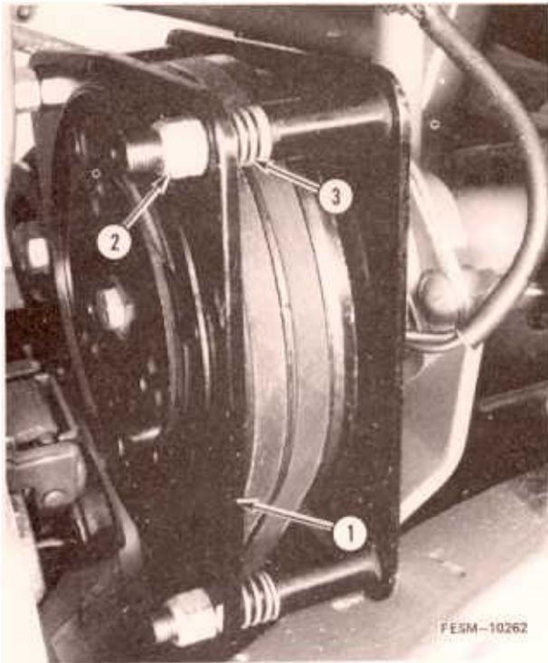
5. Remove the PTO clutch brake plate lock nuts and remove the brake plate assembly and springs and slip off the drive belts.
