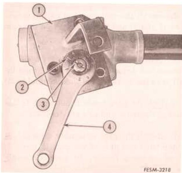
10. Install the steering gear support (1) and then install the steering arm (4) on the lever and shaft assembly. Be sure the mark (2) on the steering arm is in line with the mark (3) on the shaft. Install the steering arm nut and tighten securely.
