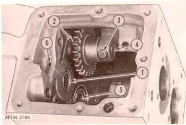
1. Spline and clutch shaft rear bearing
