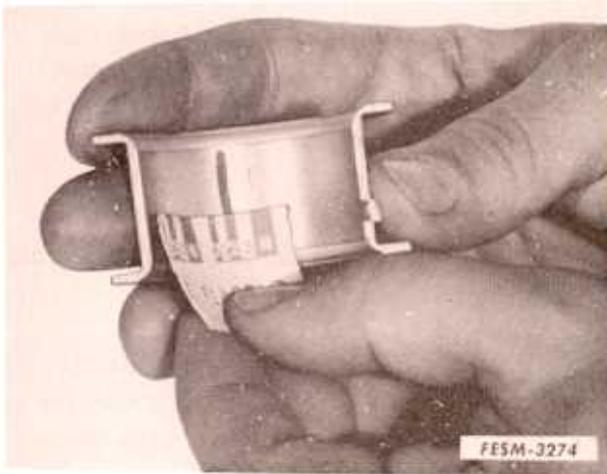
present between the bearing surface and the crankshaft journal. Measure the thickness with a micrometer or match the flattened Plastigage at several points (on either the bearing insert or the crankshaft), with the corresponding graduation on the Plastigage envelope, which indicates the clearance in thousandths of an inch. Running clearance must be .002 to .003 inch.
