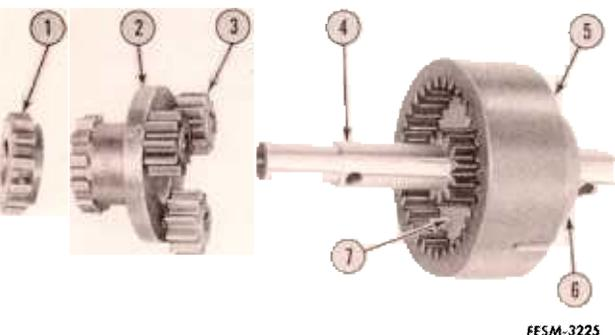
1. Direct drive spline gear
