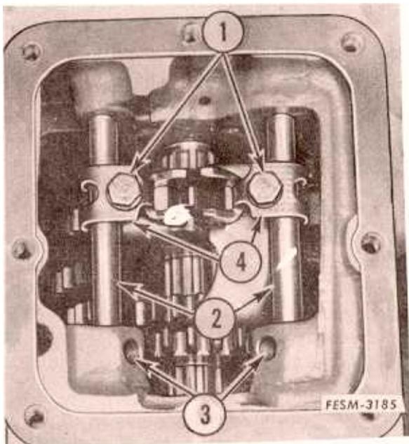
6. Shift the transmission into the neutral position and remove the shifter fork set screws (1).
