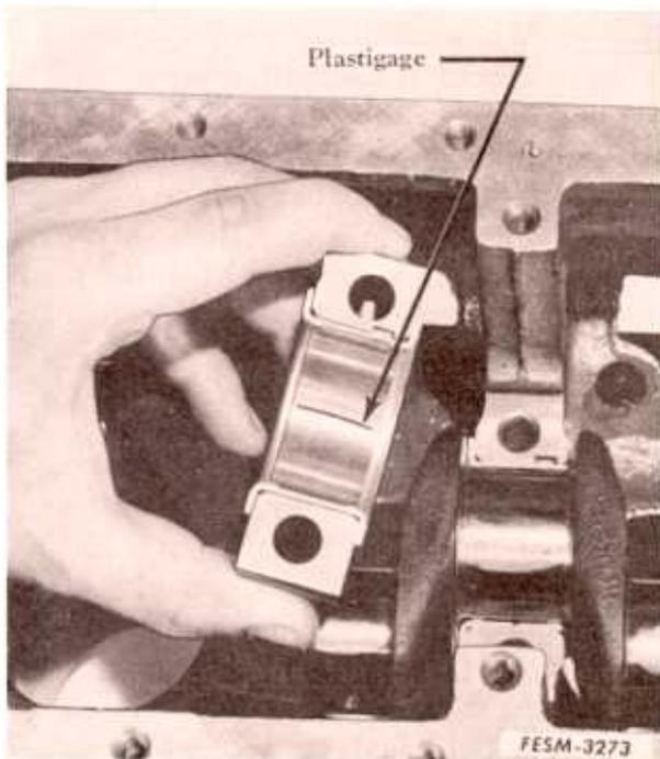
(d) Remove the bearing cap. The flattened section of the virgin lead or "Plastigage" represents the clearance
