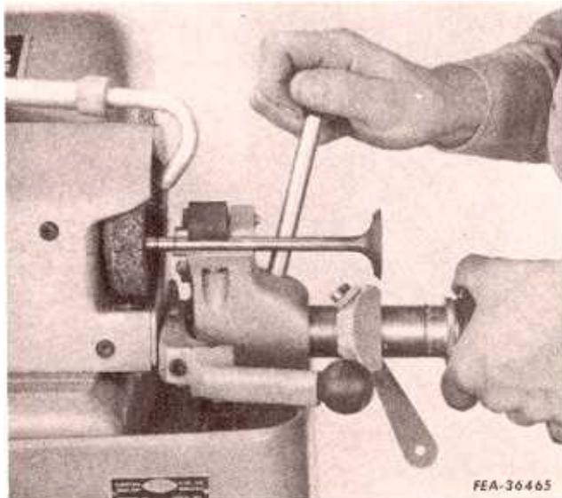
The grinding stones on both the valve refacing machine and valve seat grinder should be dressed before starting a reconditioning job.
