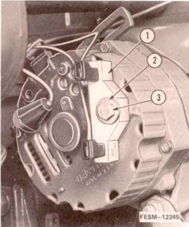
The resistor unit on the 184 tractor models, serial no. U046614 and above, requires a longer bolt and a plain washer instead of a lockwasher. The plain washer should be located between the bolt head and the resistor unit. Torque should not exceed 9-11 N·m (80-100 in. lbs.) to reduce the possibility of breakage of the ceramic resistor.
