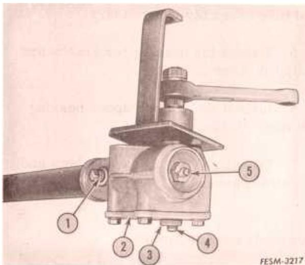
7. Install a new gasket and the side cover (2). Tighten the cap screws to 20 ft. lbs. torque.
