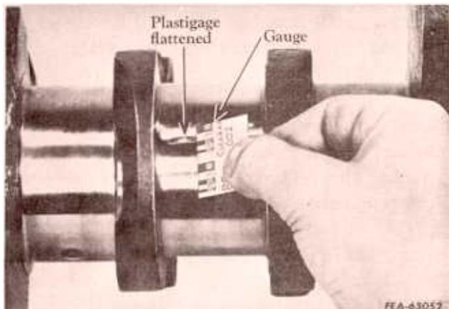
(a) Remove bearing cap and wipe bearing surface and exposed half of crankshaft journal free of oil.
