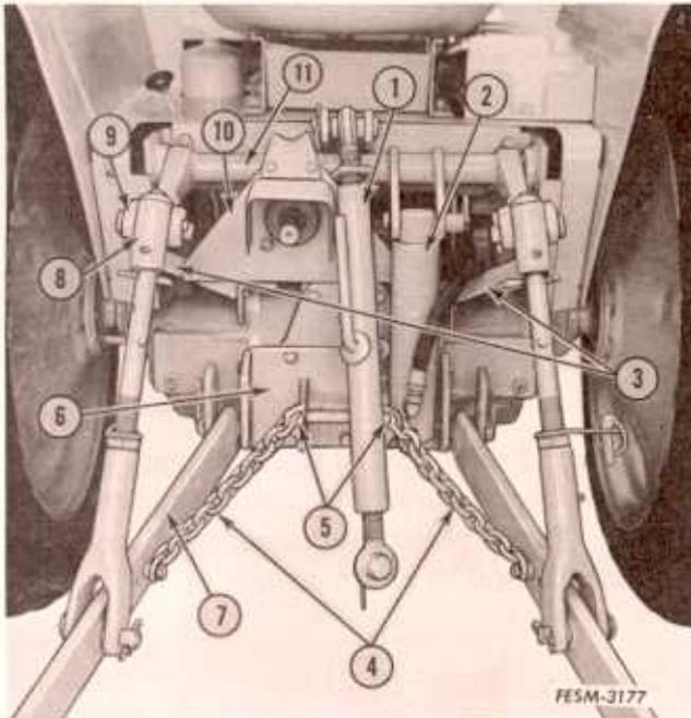
10. Remove the seat support sheet assemblies. If the tractor is equipped with three point hitch, remove the rockshaft support assembly as follows:
