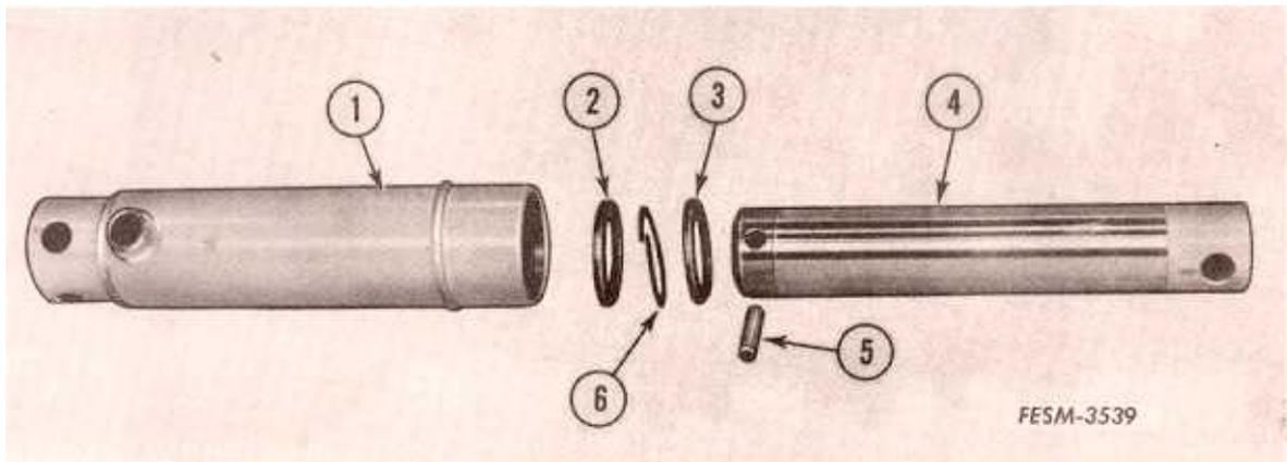
3. Remove the piston (4) from the cylinder body (1).
