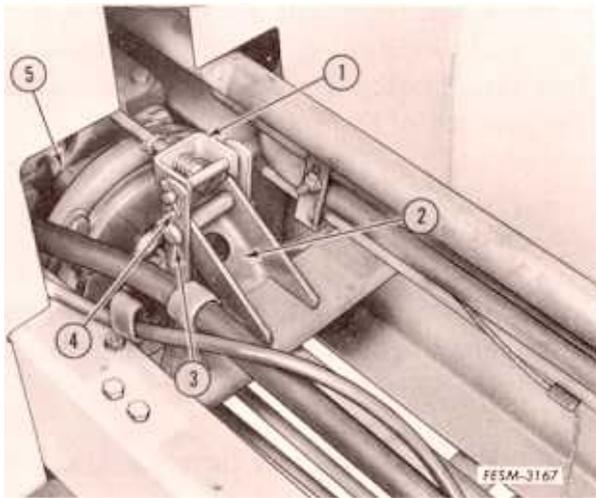
10. Remove the clutch brake yoke (1) from the clutch release yoke (4).
