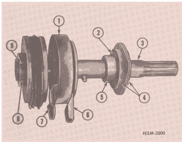
1. Loosen the bearing locking collar (5) and remove the PTO shaft rear ball bearing (2), locking collar (5) and bearing flanges (4).
