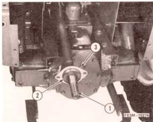
1. PTO shaft (spline end)
