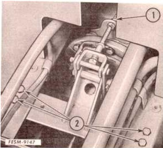
3. Remove the pin securing the clutch rod to the clutch release yoke. Remove the nut from the end of the clutch brake bolt. Remove the four bolts securing the clutch release bracket to the frame and slide the clutch release bracket ahead.
