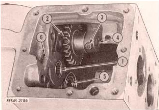
1. Spline and clutch shaft rear bearing
