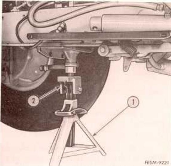
12. Support the frame of the tractor using one jack stand FES 142-4 with an adapter (2), FES 142-13 and remove the cap screws from both sides that secure the transmission case to the frame. Raise the rear of the frame to clear the axle housing.
