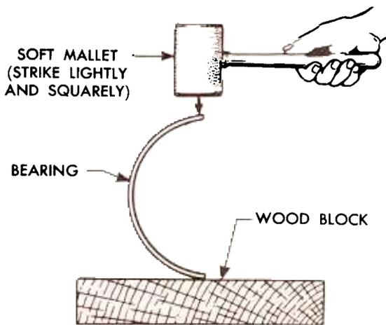
(a) **EXCESSIVE SPREAD:** If measurement of bearing indicates that dimension "A" is excessive, place bearing on a wood block and strike the side lightly and squarely with a soft mallet. Recheck measurement and, if necessary, continue until correct width is obtained.
