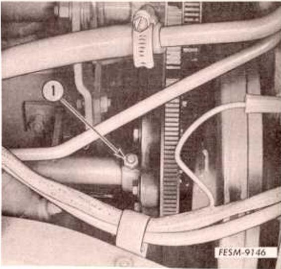
2. Remove the Allen head bolt from the clutch shaft coupling and slide the shaft ahead.
