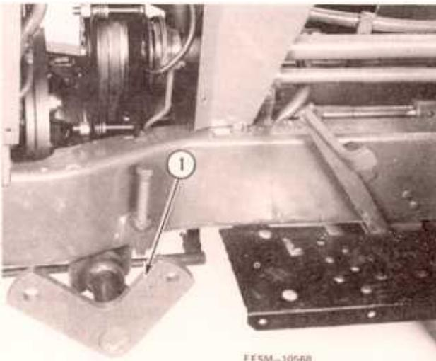
7. Remove the rockshaft from under the tractor.
