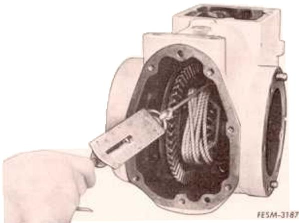
9. Check bearing preload before installing the transmission countershaft. Preload is correct when a steady pull of one to eight pounds is necessary to rotate the differential assembly.
