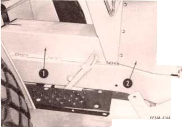
1. Remove the frame top cover (1) and pedestal side sheet sections (2).
