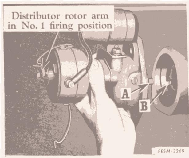
9. Position the ignition unit distributor arm and drive shaft lug (A) for firing number one cylinder. Install the ignition unit on the engine, meshing distributor lug (A) and governor drive slots (B).
