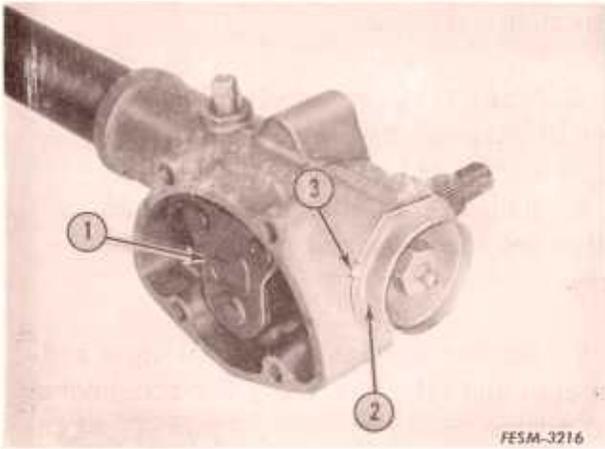
5. Install the lock nut (2) and tighten securely. Stake the nut into a housing slot (3).
