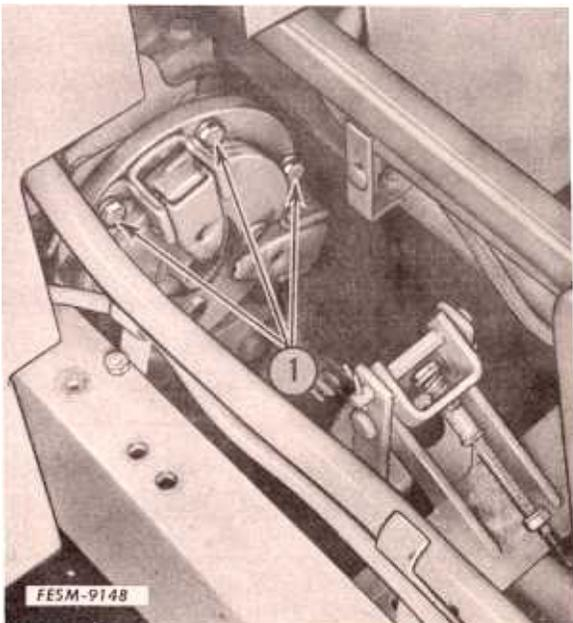
4. Remove the six bolts securing the pressure plate assembly to the input flywheel. Remove the pressure plate assembly and the clutch disc.
