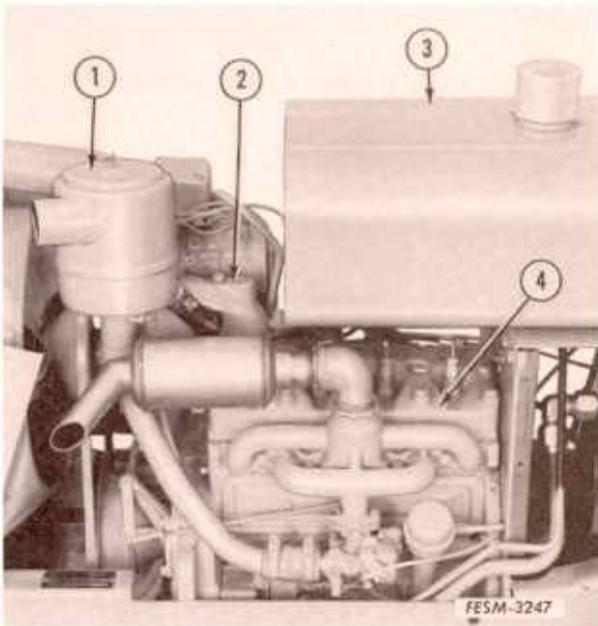
1. Remove the pipe plug in the water inlet elbow and drain the coolant.
