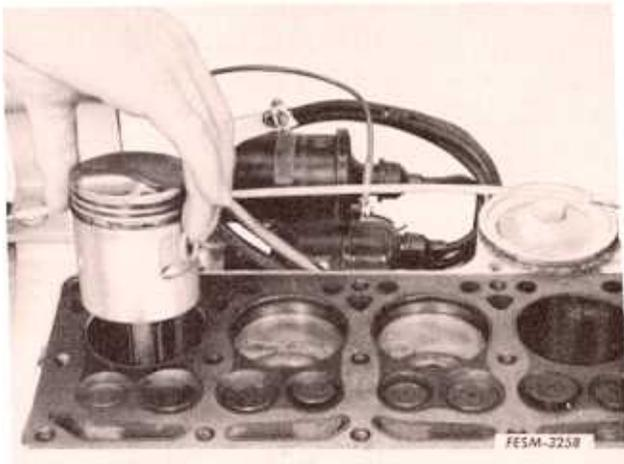
6. Push the connecting rod and piston assembly to the top and lift out from the crankcase. Replace the cap on the connecting rod to avoid damage.
