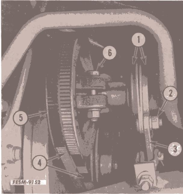
6. Install the second bearing flange (1) on the shaft. Place the PTO driven pulley (5) in position and move the drive shaft into it. Install the retaining snap ring or bolt.
