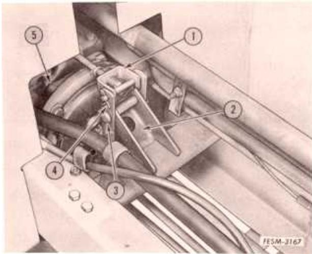
8. Install the pin securing the clutch brake yoke (1) to the clutch release yoke (4).
