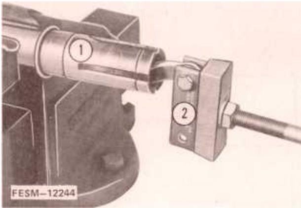
9. To remove the innermost bearing, use a slide hammer with only one appropriate length leg as shown.
