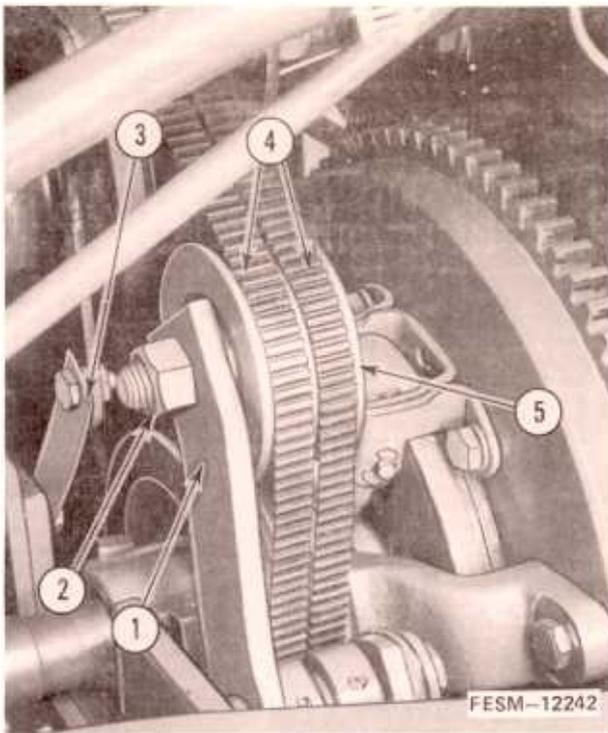
15. Relieve the IPTO clutch belt tension by pushing in on the idler tension arm nut with a 3/4 inch wrench and then remove the drive belts from the tension arm pulley.
