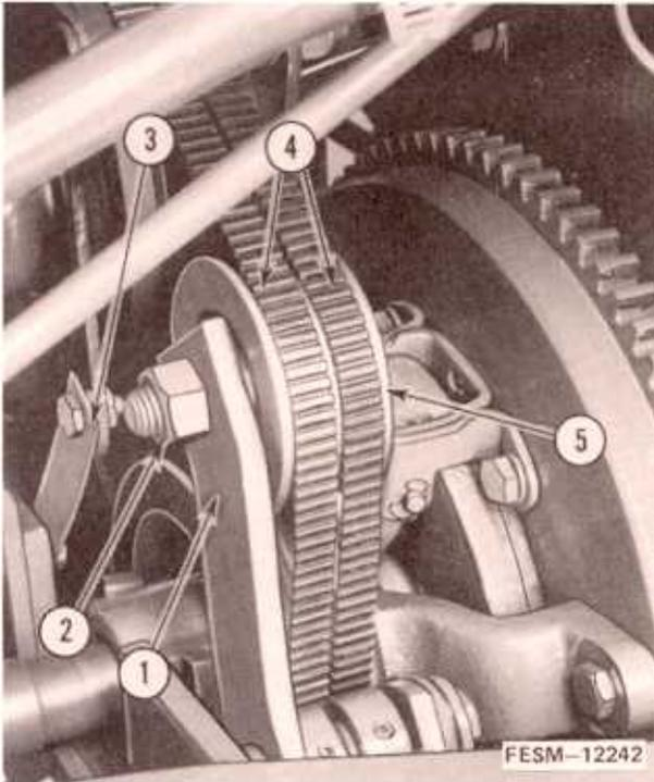
3. Relieve the clutch belt tension by pushing in on the idler tension arm nut with a 3/4 inch wrench and then slip the drive belts off the tension arm pulley.
