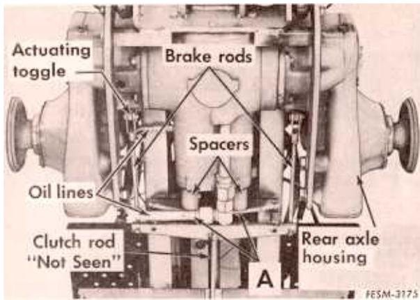
2. Remove the two cap screws (A) and spacers' (no spacers w/creeper drive) securing the front of the transmission to the frame.
