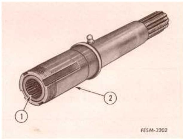
8. If needle bearings are to be replaced, remove the outermost bearing using a slide hammer with two legs.
