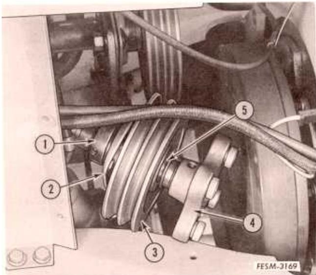
20. Move the front of the shaft over the flywheel and remove the clutch coupling (4), snap ring (5) and pulley (3).
