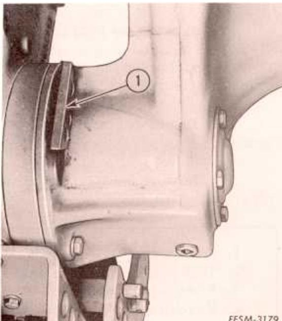
1. Be sure to install the reinforcement block (1) on the R.H. final drive assembly if it was removed.
