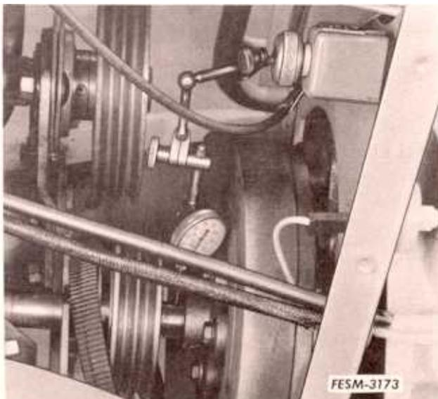
d. Tap the coupling in the direction required to reduce run-out to minimum possible.
