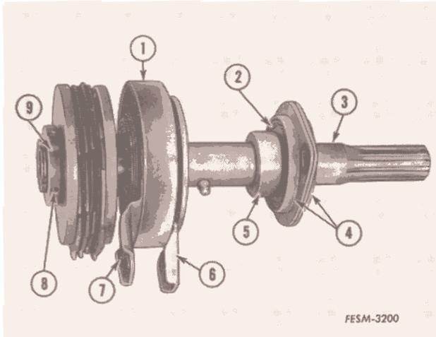
10. Install the bearing flanges (4), locking collar (5) and shaft ball bearing (2). Do not tighten the locking collar at this time.
