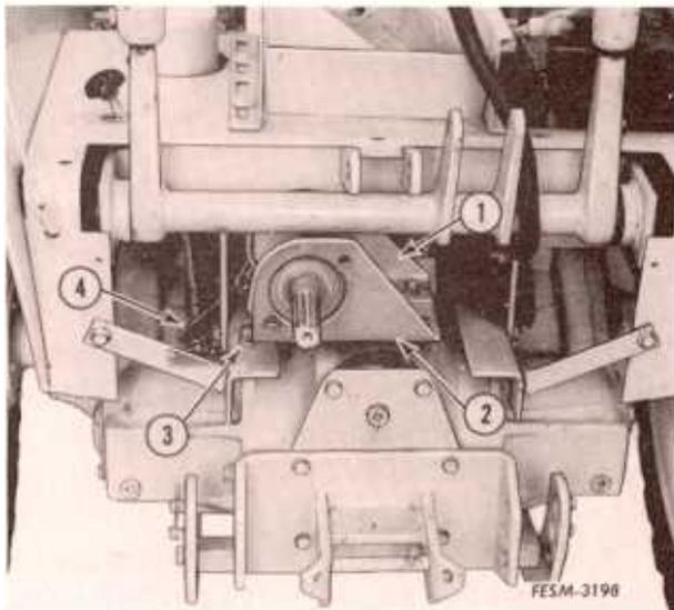
12. Connect the clutch control arm (4) to the actuating cam.
