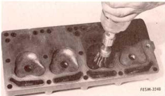
1. Check the head and gasket for "blow-by" or compression leaks.
