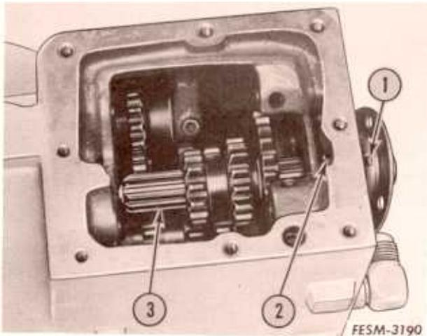
1. Shaft oil seal slot
