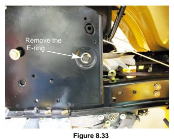
Deck lift shaft assembly bushings
