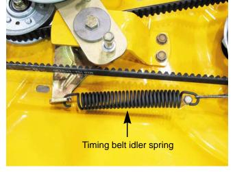
5. Remove the timing belt idler spring. See Figure 8.25.
