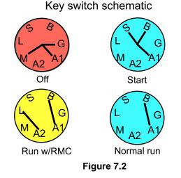
position. Check continuity from yellow wire connection all the way to the spade terminal on the magneto.
