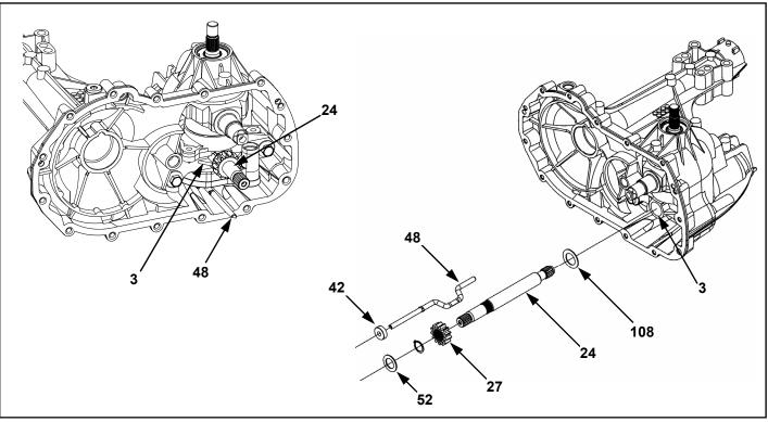
Figure 13. Motor Shaft & Bypass Rod Assemblies
