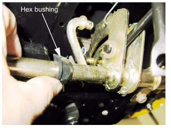
4. Slip the tie plate off of the hex bushing, and remove it.
