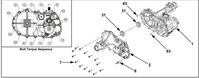
Figure 11. Side Housing Assembly
