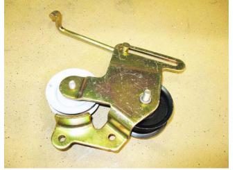
Maneuver the belt tensioner bracket assembly to clear the belt, and remove it from the tractor. See Figure 5.39.
