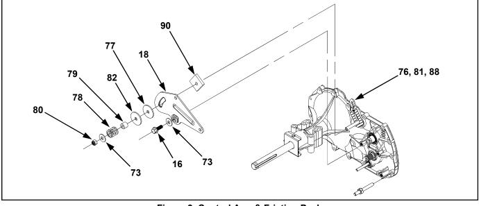
Figure 9. Control Arm & Friction Pack
