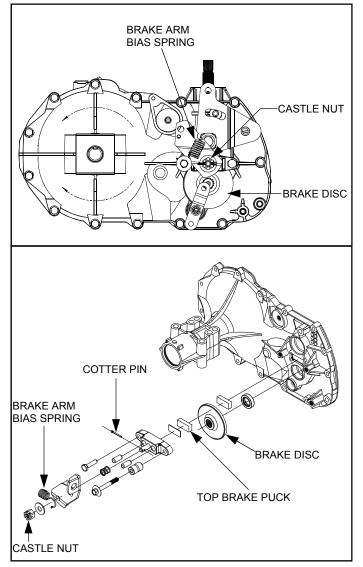
Figure 6. Brake Components
