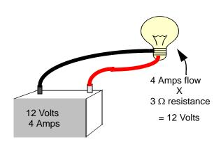
As an example, imagine a circuit that has a 12V battery that produces 4 amps of current powering a light bulb that creates 3  $\Omega$  of resistance. The wires are assumed to have 0  $\Omega$  resistance\*. The light bulb uses 12 volts (4 amps x 3 ohms = 12 volts). The battery produces 12 volts that equals the 12 volts used by the light bulb. See Figure 7.47.
