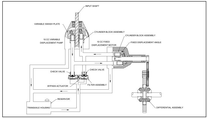
Figure 2. 310-0510 Hydraulic Flow Illustration
