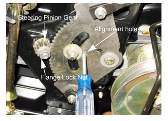
4. Remove the flange lock nut securing the steering pinion gear to the steering shaft using an 11/16" socket. See Figure 3A.17.
