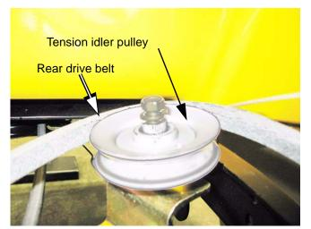
4c. Lift the pulley far enough to allow the belt to clear the belt keepers. See Figure 6.61.
