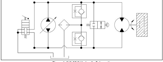
Figure 1. 310-0510 Hydraulic Schematic
