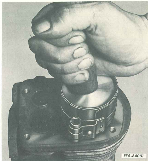
Illust. 11. Installing piston assembly.
