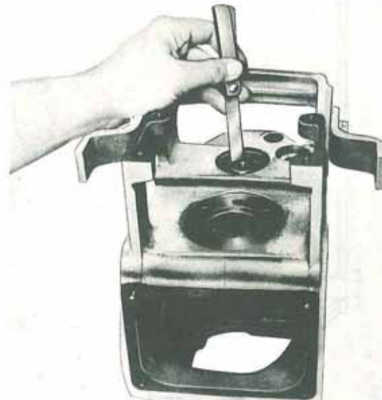
Illust. 2-49. Measuring snap ring groove gap.
