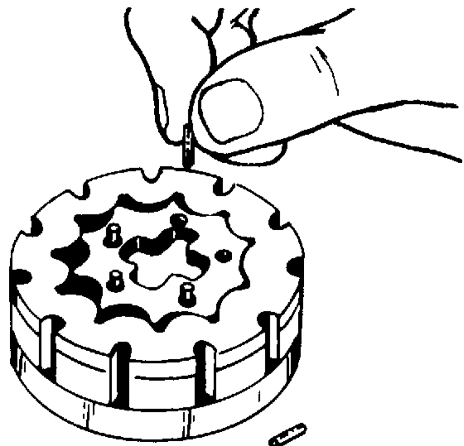
Figure 4-28. Removing Needle Rollers.
